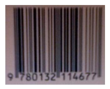
The encoded digit string, 9780132114677, is printed below the barcode. The left group encodes the digits 780132, with 9 encoded in their parity. The right group encodes the digits 114677, where the final 7 is the check digit. Here's a clean encoding of this barcode, from one of the many web sites that offer barcode image generation for free.
