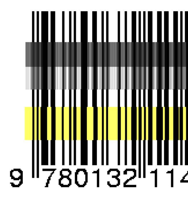
The luminance-converted row from the photo is in the dark grey band. It is low in contrast and poor in quality, with plenty of blurring and noise. The paler band is the same row with the contrast adjusted.
